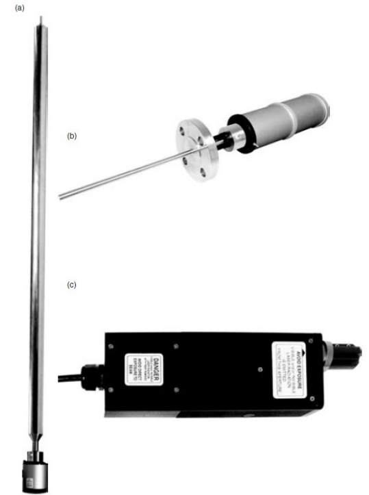
Figure 5.4 Collection of commercial Raman probes designed for different installations: (a) fifteen-foot immersion probe; (b) typical immersion probe, approximately one-foot long; and (c) probe body for a non-contact probe with fitting to accept different focal length optics. Adapted, with permission, Copyright © 2004 Kaiser Optical Systems, Inc.
